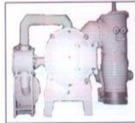
Vacuum heat treatment equipment
